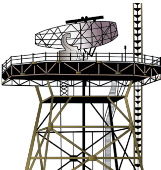
Figure 9-7. Combined Radar and Beacon Antenna.
