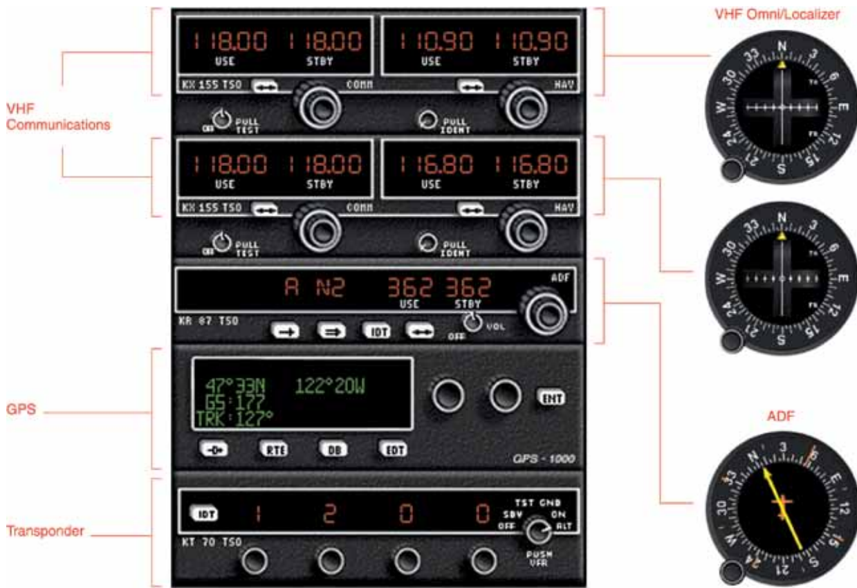
Figure 9-1. Typical NAV/COM Installation.
